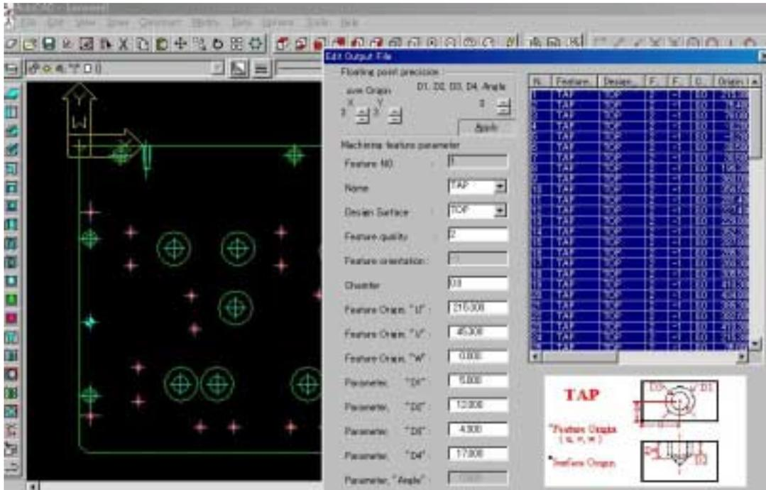
Fig. 7. Example Product Data automatically analyzed by the FR capability and presented for confirmation or modification by the user.
