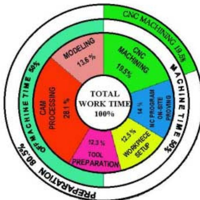
Fig. 18. Percentage share of work time among preparatory and machining tasks for making a first piece of a product component.
