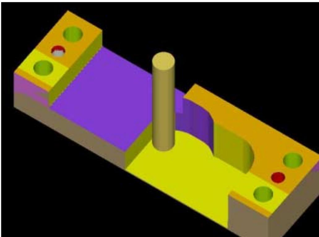
Fig. 10. Graphic simulation of the tool motion by commercially available software, Super Verify (<http://www.aikoku.com/aec/index.htm>)
