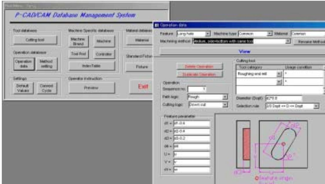
Fig. 11. Main database dialog box and the example viewing of the operation database.
