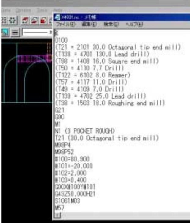
Fig. 9. Example NC program generated by P-CAD/CAM software and ready for uploading to the MC assigned for the job.
