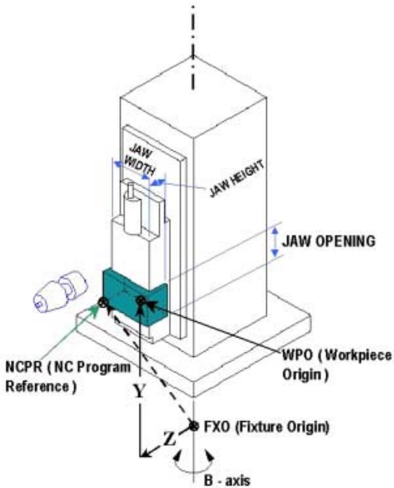
Fig 12. Three faces machining by horizontal machining center.
