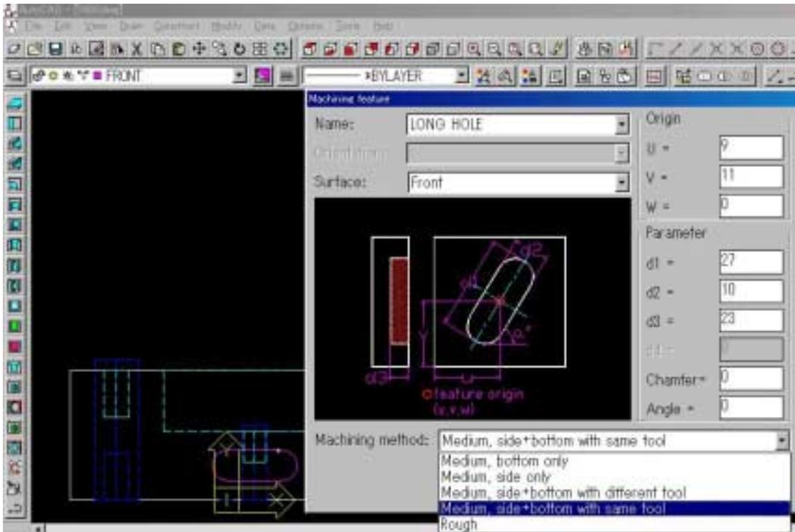
Fig. 4. Machining feature design dialog box.
