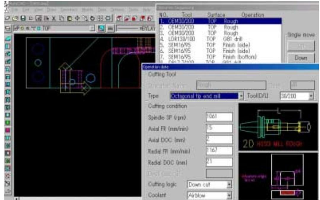
Fig. 8. Example operation details presented by the CAM software for confirmation and/or modification by the user.
